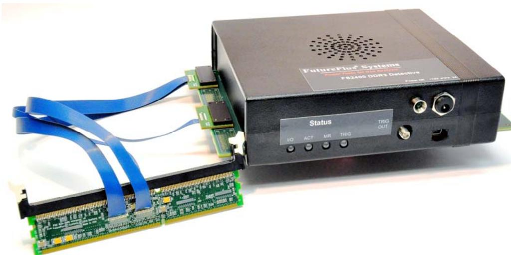
**Figure 9:** The *DDR3 Detective*<sup>™</sup> unit cabled to the DDR3 DIMM interposer.
