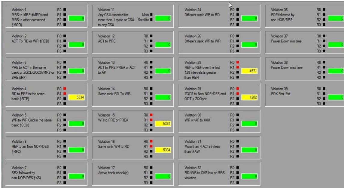
**Figure 1:** Protocol Compliance Violations found in our system under test. Red indicates failing Rank, yellow indicates number of failures
