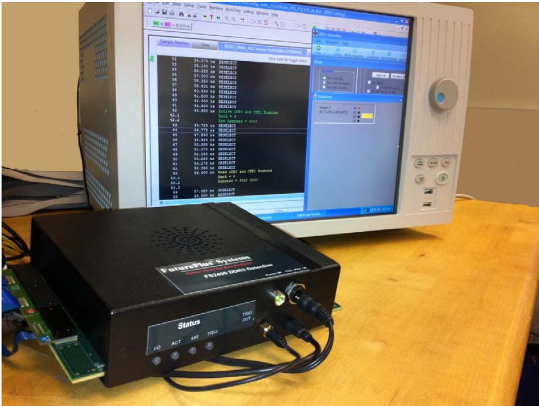
**Figure 8 :** When used in conjunction with a logic analyzer the *DDR3 Detective*<sup>™</sup> can show the DDR Data bus traffic around the error in addition to the Address/Command/Control signals.
