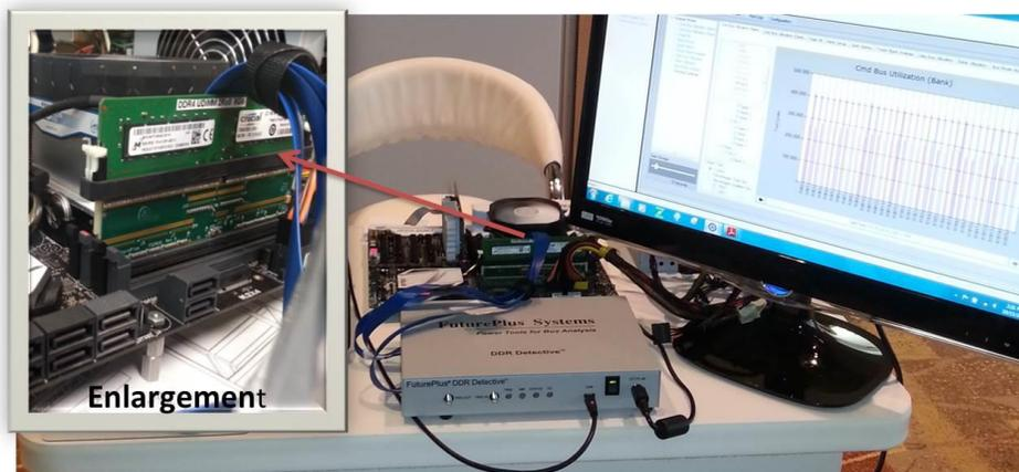
Figure 1: DDR4 Memory Performance Metrics illustrated on an ASUS X99 System using the DDR Detective® from FuturePlus Systems
