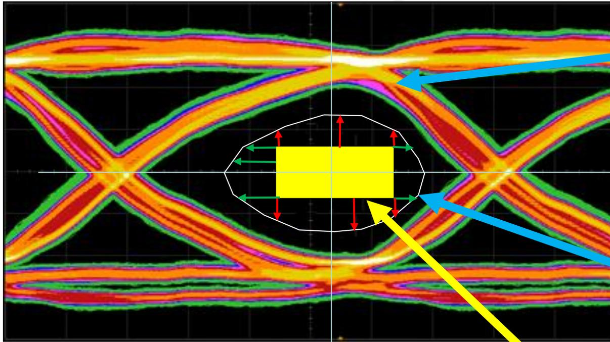
About 1E6 bits accumulated by scope at DRAM pin
